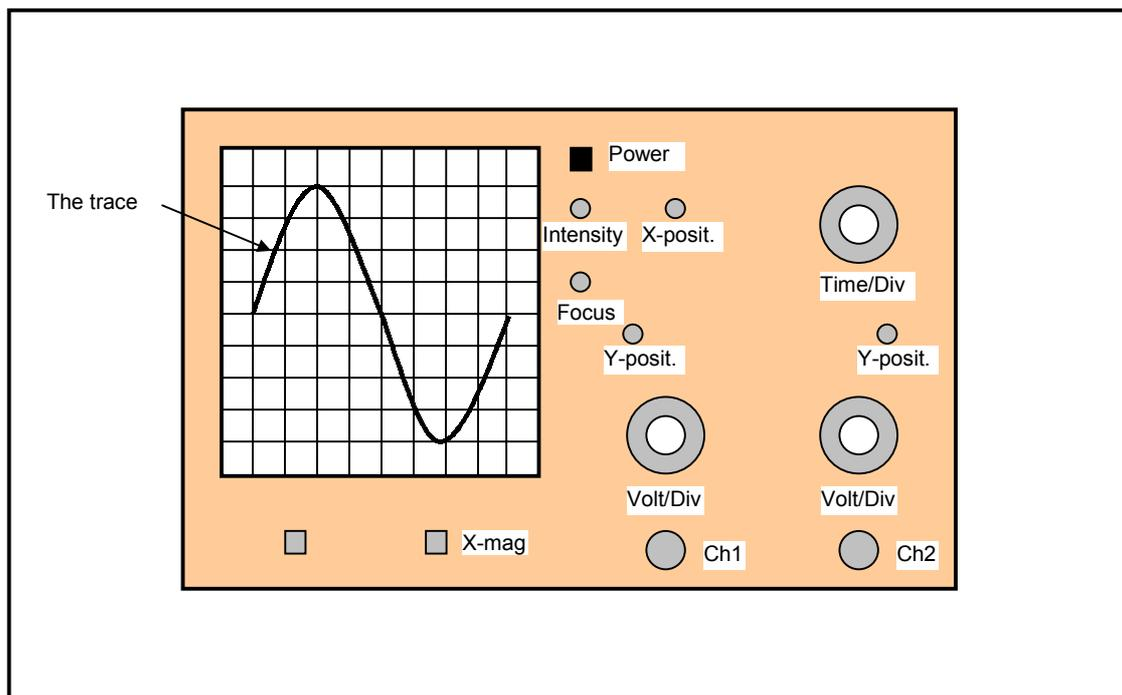
**Figure 2:** The front panel of the *CRO*
