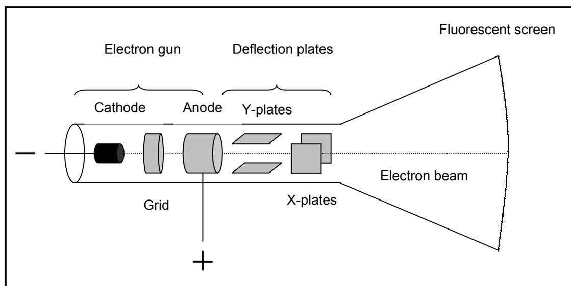
**Figure 1:** The basic structure of a CRO
