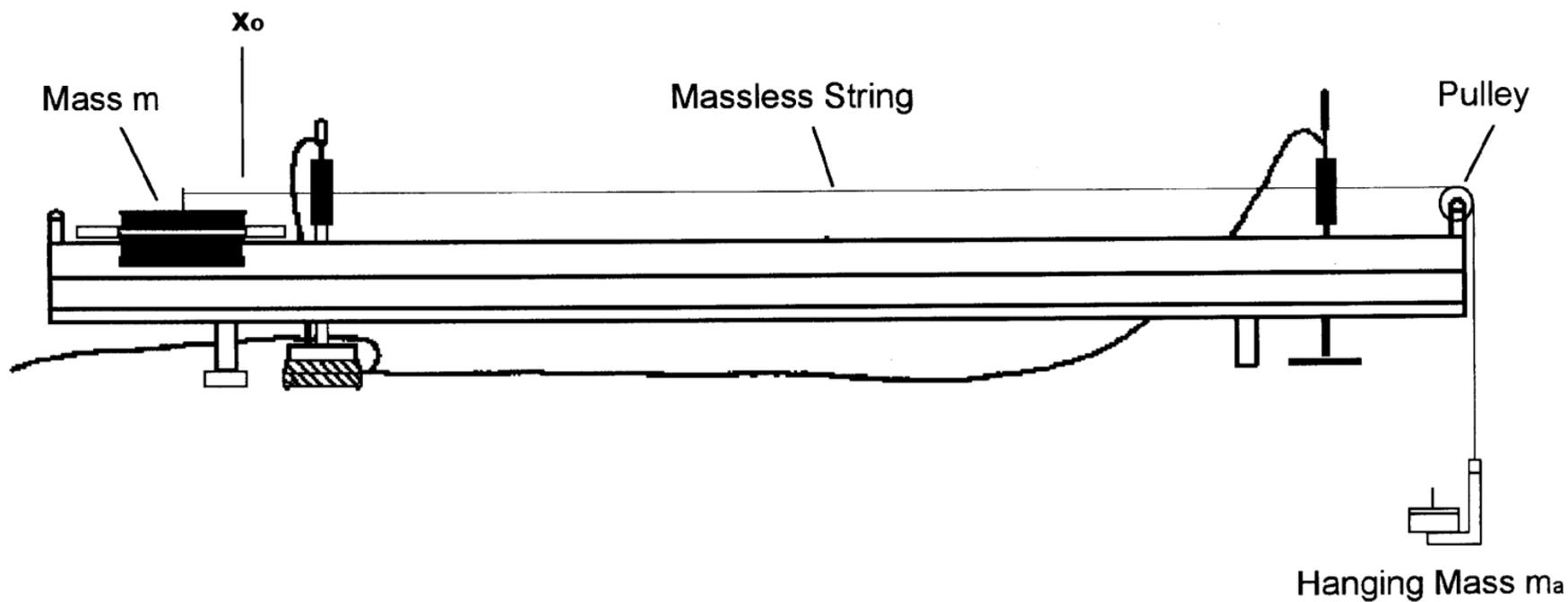
Figure 9 : Experimental Setup for Part B " Newton's Second Law"
