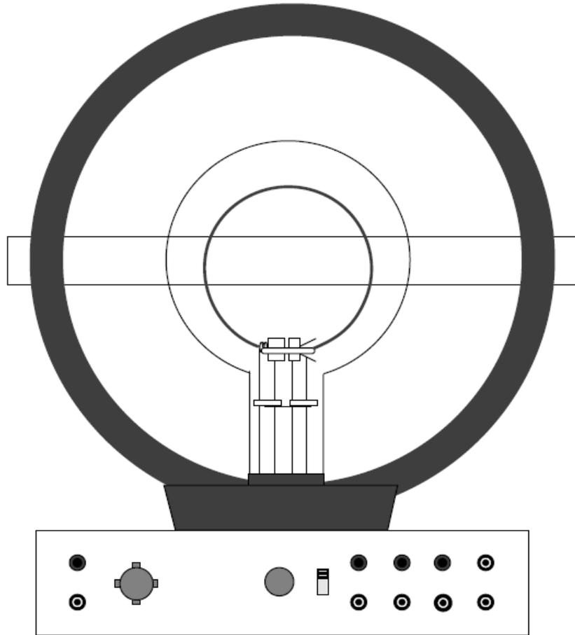
Figure 3. The  $e/m$  Apparatus
