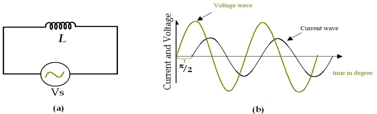
**Figure 1.** (a) schematic diagram of purely reactive circuit
