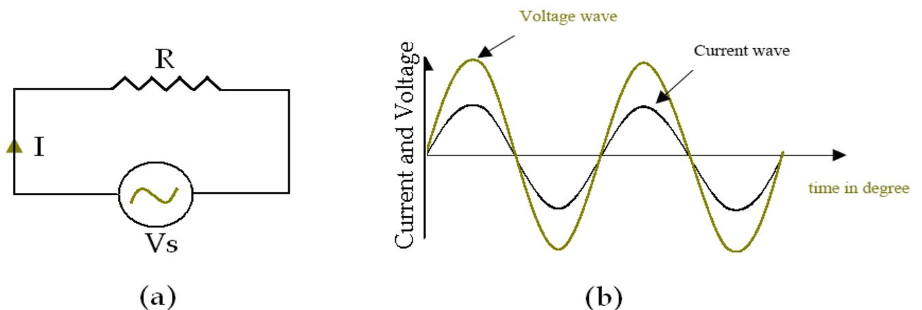
**Figure 2.** (a) schematic diagram of purely resistive circuit
