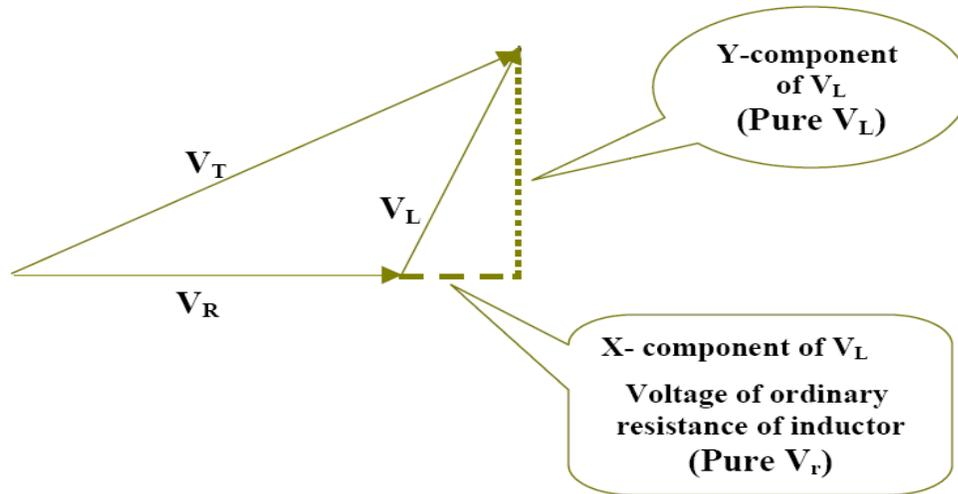
**Figure 4.** Phase diagram between  $V_L$ ,  $V_R$ , and  $V_r$ .
