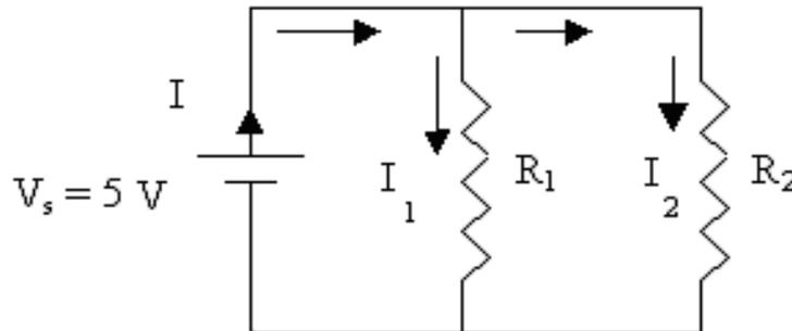
**Figure 3.** Two resistors connected on parallel to the voltage source.
