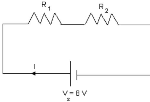
**Figure 2.** Two resistors are connected end-to-end (series)
