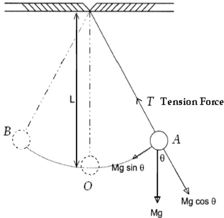
**Figure 2.** Simple Pendulum
