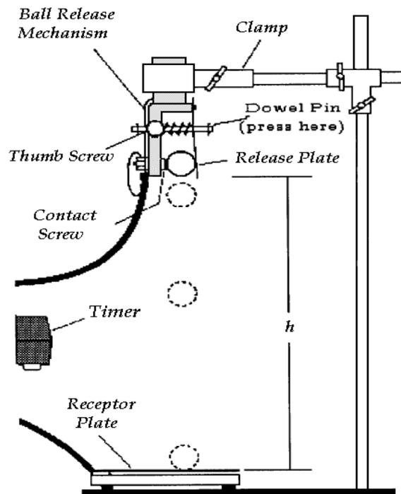
Figure 1 Free Falling Apparatus
